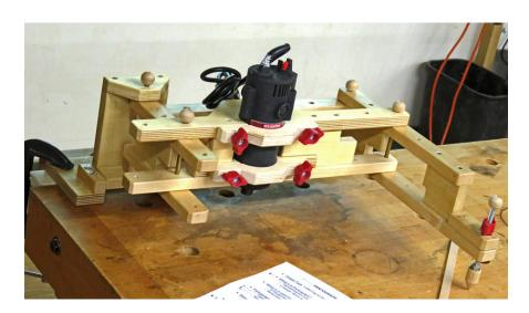
So, the \$64 question is, "How did it perform?". In limited testing, Paul noted that the tool performed up to expectations. The only anomaly that surfaced was that, due to the vibration of the router and the slight taper on the ends of the rods, some of the pivot rods tended to work themselves out of their holes. To prevent that, he drilled and tapped the ends of the pivot rods and installed small screws and washers – problem solved.
