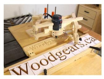
The **Woodgears.ca** router pantograph design appeared to be very simple to build with commonly available materials and shop equipment. Also, as illustrated on the website, the tool appeared to be ideally suited for lettering signs, a feature which was of interest for **Paul's** box engraving application.
