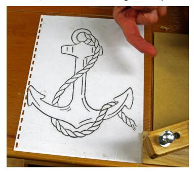
Working carefully, he traced the pattern outline with the tapered Stylus. The router bit he used was a 1/4" diameter, **solid carbide**, sign making bit, with a **15**º included angle tip.
