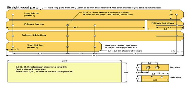
The **Woodgears.ca** router pantograph design is unique in that it utilizes a *hinged* fixed pivot mount, allowing motion in the *vertical* direction, enabling it to do **3D copying**. The **Woodgears.ca** website has some very interesting photo documentation showing the routing of a 3D shape.
